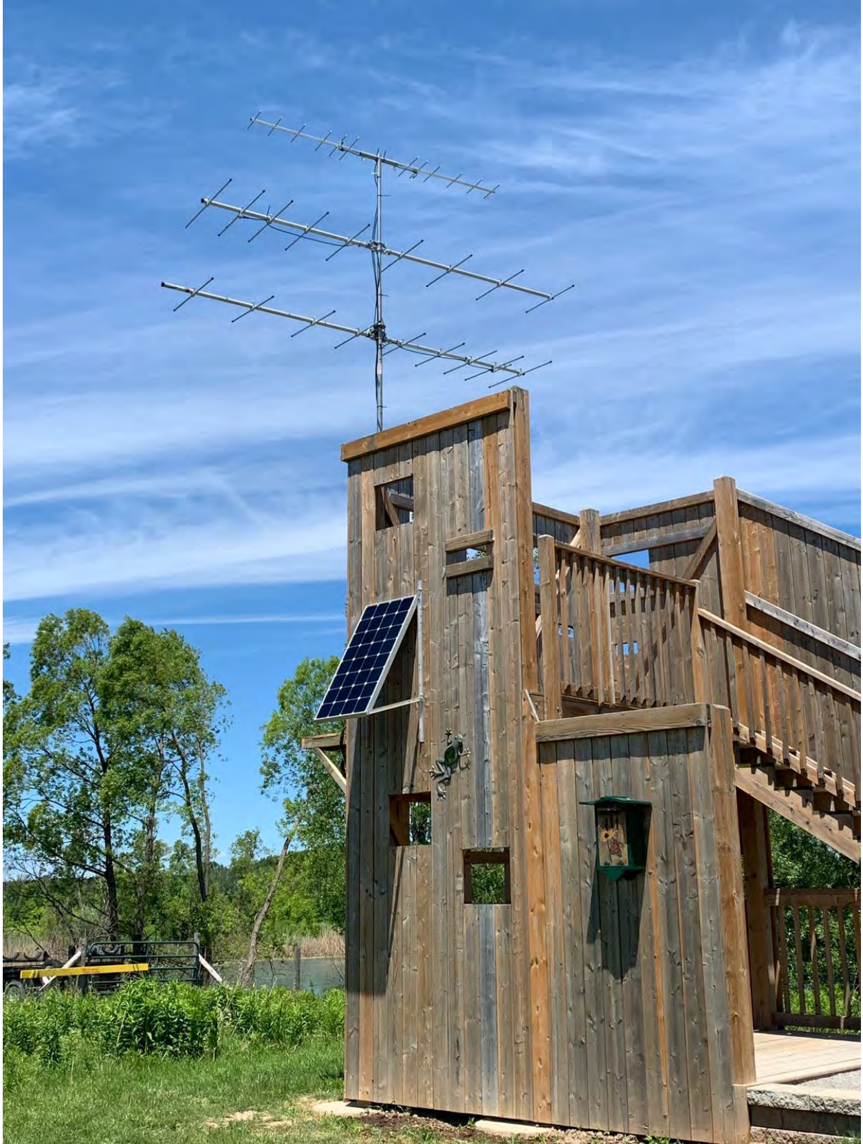
Motus station mounted on viewing platform at Grimsby wetland, ON.
