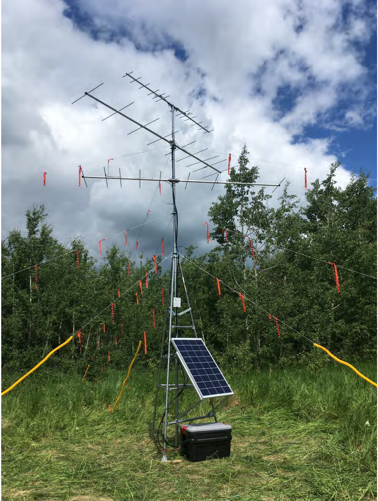
Solar-powered pop-up tower Motus station in Dawson Creek, BC.
