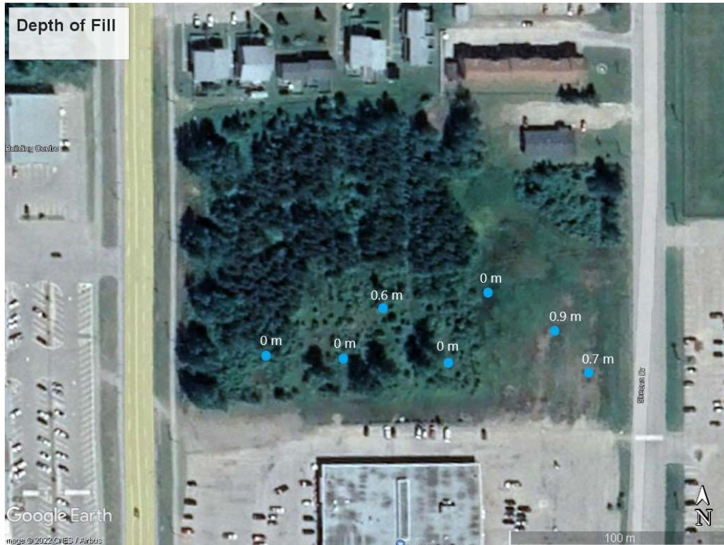
Figure 2. Depth of fill/disturbed soil in test pits shown on Google Earth Imagery.
