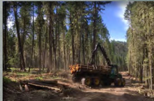
FIGURE 3: Forwarder with a turn of logs to roadside.
